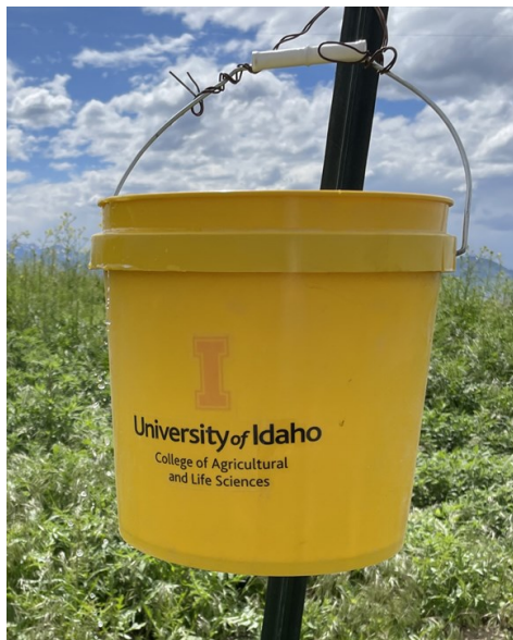
Figure 2. Two-gallon yellow bucket water trap. These traps are typically positioned along field edges, ideally in areas with visible soil and weed control. They are filled to the brim with water, a drop of soap is added to break surface tension and prevent aphids from escaping, and a few crystals of copper sulfate inhibit algae growth. The contents are collected weekly and taken to our Idaho Falls lab for aphid counting.
