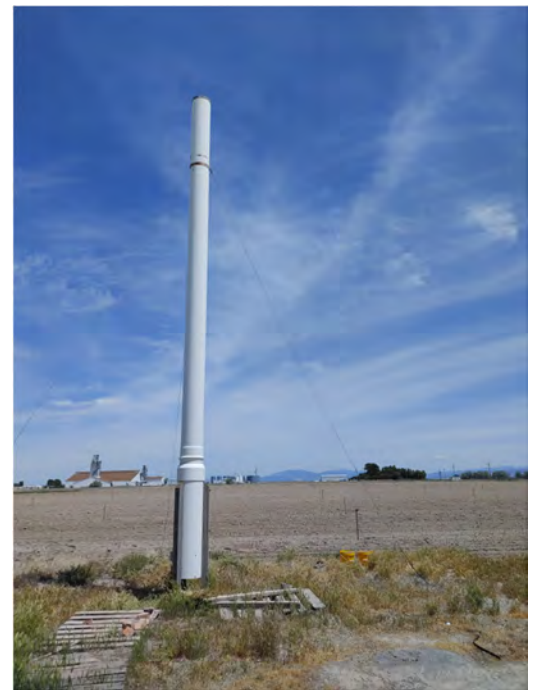
Figure 1. Tall, fixed suction trap at the Aberdeen Research & Extension Center in Aberdeen, Idaho. This trap was part of a larger aphid monitoring network that operated statewide from 1985 to 2003.
