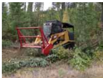
Figure 39. Mechanical slash reduction typically involves some type of attachment to an excavator, a bobcat, caterpillar, or similar machine.
