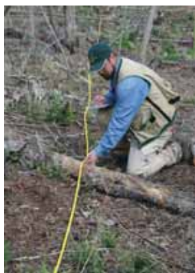
Figure 69. CWD can be measured using transects.
