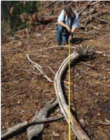
Figure 72. If the same piece crosses the transect more than once it is counted each time.
