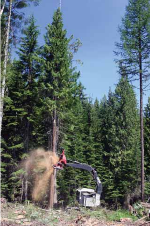
A harvester leaving a snag and removing the merchantable part of the tree.
