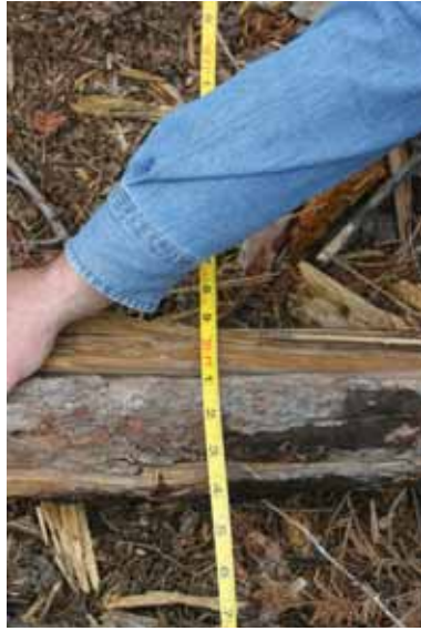
Figures 71. Splintered logs are mentally molded together to estimate diameter – this piece would be roughly 5 inches.
