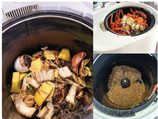
Figure 3. Electric food cyclers dry and grind food waste into a pre-compost product.
