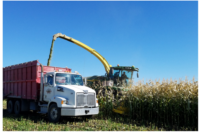
Figure 2. Corn for silage being harvested by a self-propelled forage harvester.
