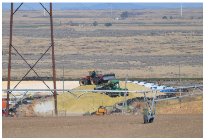
Figure 3. Two large packing tractors are needed to pack down a silage pile because significant machine weight is critical to ensure good quality silage.
