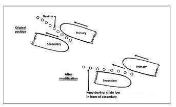
**Figure 5**. Modifying the position of the deviner chain so that it rests on the secondary conveyor reduces tuber damage.
