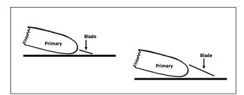
**Figure 4**. Angling the digger blade into the front of the primary conveyor (left) jams tubers into the chain. Aligning the blade tangent to the primary (right) causes less bruising.
