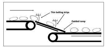
**Figure 7**. A cushioned ramp reduces the impact force experienced by potatoes as they move between conveyors.
