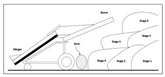
Figure 6. Piling potatoes in stages reduces bruising due to rollback on the face of the pile.
