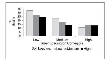
**Figure 3**. Relative bruise level when chains are full of soil or tubers (high) versus medium or low loading on the chains. Redrawn from Hyde G. M., R. E. Thornton, J. A. Francis, and R. E. Hermanson. 1990. "Potato Harvester Chain Speed Adjustment." Extension Bulletin 1558. Washington State University.
