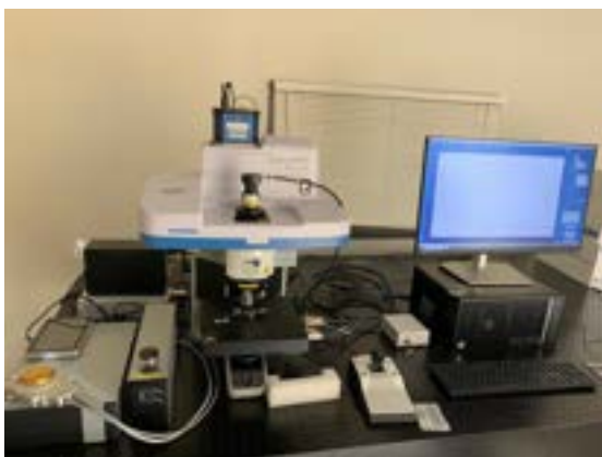
Confocal Raman Microscope (Horiba, XploRA Plus) with a Linkam Hot stage. Raman spectra can be obtained in-situ while heating the samples to 1100 °C
