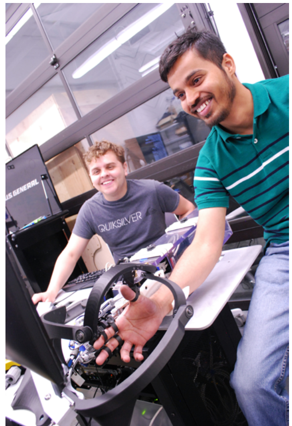
(Above) Graduate students Chris Bitikofer (left) and Rene Maura (right) test the a dual-arm exoskeleton BLUE SABINO, designed to evaluate neurological impairment after stroke and gather quantitative data to refine therapeutic medicine and improve treatment.
