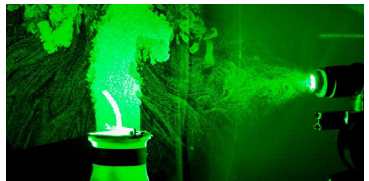
Flow visualization experiments showing the fluid flow over the flexible membrane.
