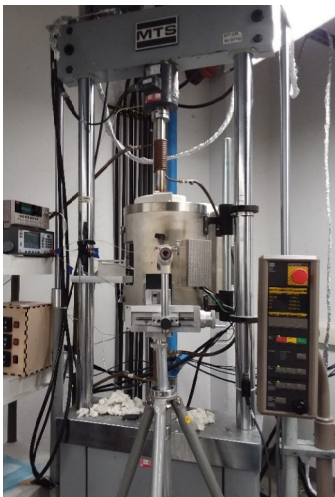
A testing frame for creep-fatigue crack growth is shown, capable of measuring crack face openings and crack growth rate.
