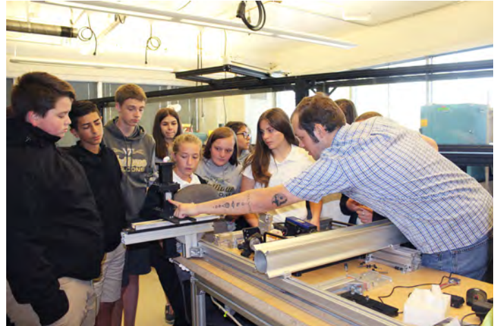
(Above) Doctoral candidate Brandon Hilliard shows visitors how the the Aquatic Imaging Flume works. (Left) The system use Particle Imaging Velocimetry and other optical measurement techniques.
