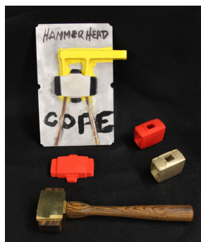
Replica of the Studley Infill Hammer. Also shown is the cope used to cast the bombe brass housing, the 3D printed pattern for the casting, and 3D mock-up of the housing.
