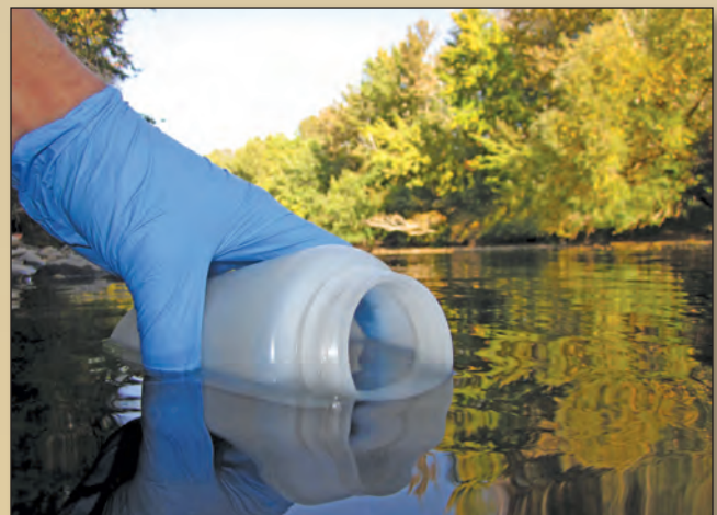
Figure 2. A water sample can be collected easily in the field in a sterile bottle and, if needed, stored temporarily in a cooler or refrigerator before eDNA is concentrated through filtration or centrifugation. Photograph taken by Matthew Laramie, U.S. Geological Survey.
