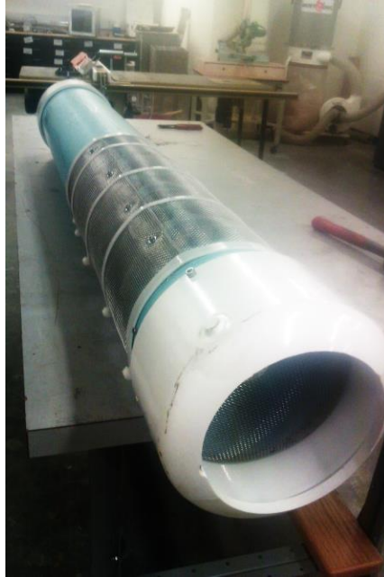
Figure 8. Pump shroud for submersible pump.
